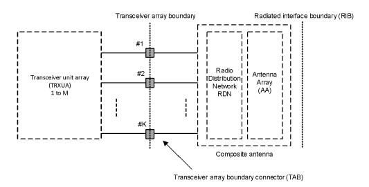
The transceiver unit array is part of the composite transceiver functionality generating modulated transmit signal structures and performing receiver combining and demodulation.
